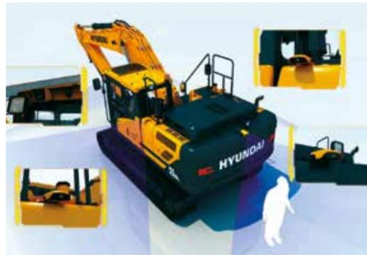
\* AAVM (Advanced Around View Monitoring): Secure field of vision in all directions by nine views including 3D bird's eye view and 2D/4CH view.
