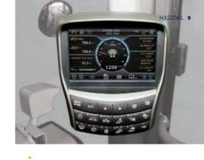
The instrument panel is optimised to provide quick, easy access to machine status information as you work. It features an 8-inch touchscreen monitor for excellent legibility.
