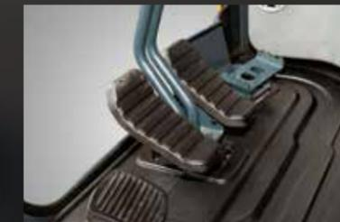
The foot rest, attachment pedal, left and right travel pedals and boom swing pedal are configured for convenient access.
